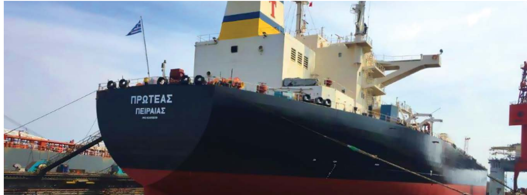
PCT Vessel - Ice Class, WorldWide L x W: 249.9m x 44m, Gross tonnage (GRT): 66.919 t, Deadweight (DWT): 117.055 t DRY DOCKING - AntiFouling System for 60 month protection - Spot Blasting Sa2 30%
